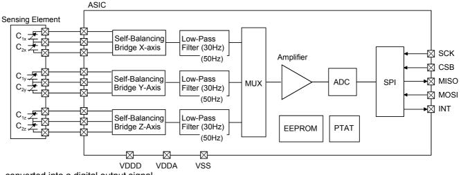
converted into a digital output signal.
